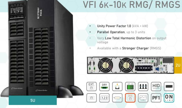
The PowerWalker VFI 6k-10k RMG PF1 is a professional UPS for commercial applications featuring Unity Power Factor (PF=1.0) and strong charger with adjustable current. The wide input voltage and frequency ranges allow operation in unstable networks and provides generator support.
